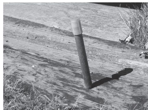
Fusee, used by railroaders to signal emergencies to oncoming train
